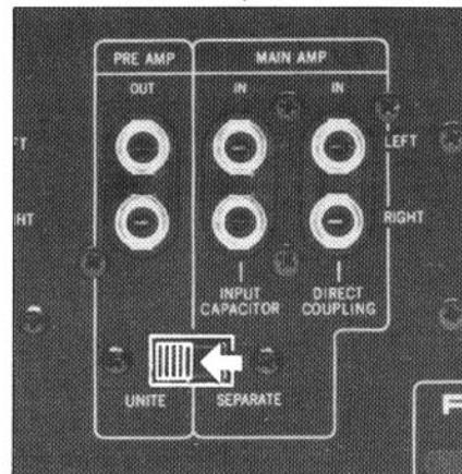
The RA-2040 is equipped with 2 types of input terminals, the 'Direct Coupling' terminal, and the 'Input Capacitor' terminal. Use the 'Direct Coupling' terminals when connecting the RA-2040 to the Rotel RC-2000 or RC-5000.
